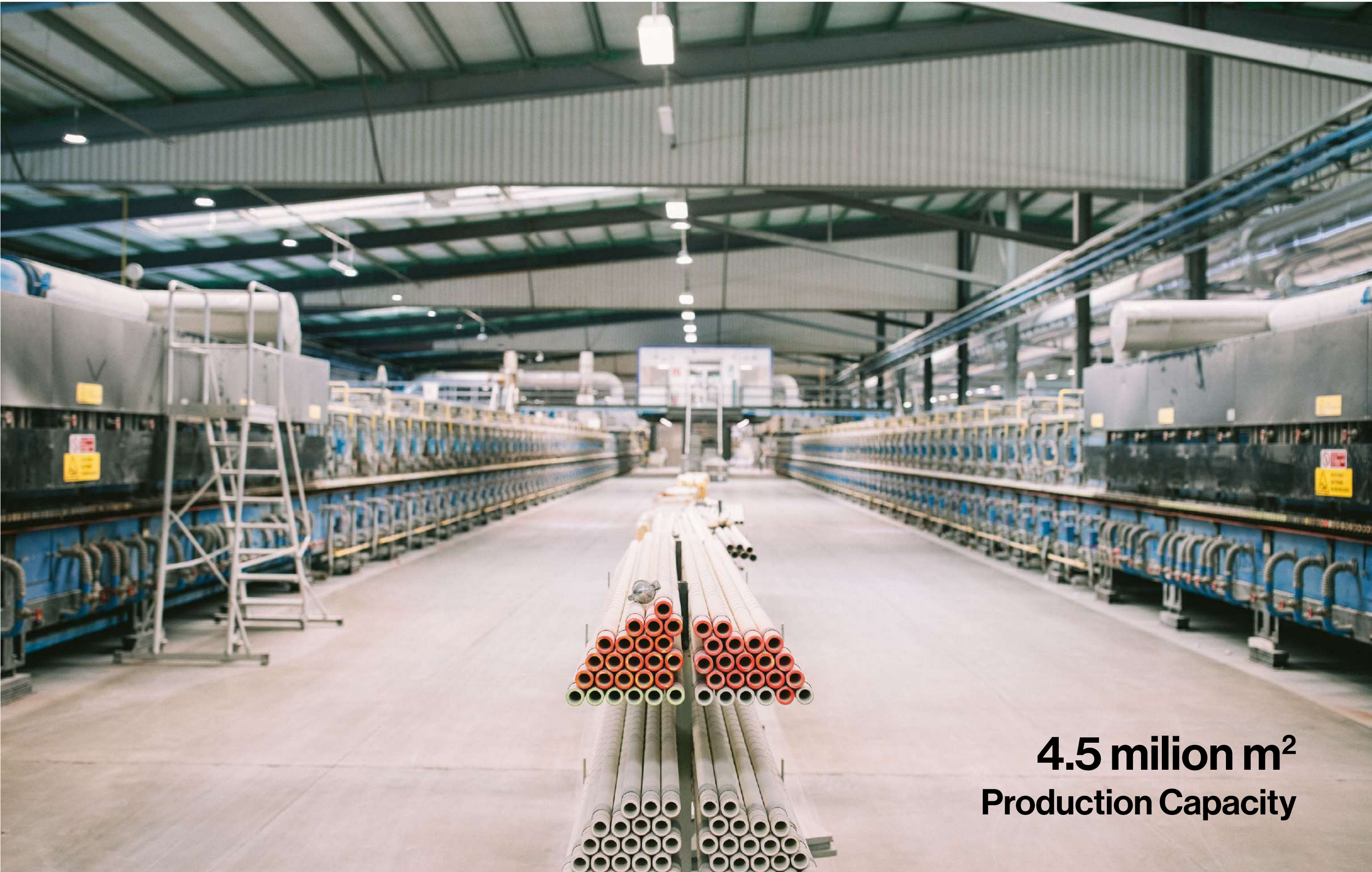
Ceramic rollers on which our porcelain slabs run through the kilns at our production site in Vetschau (Germany).
